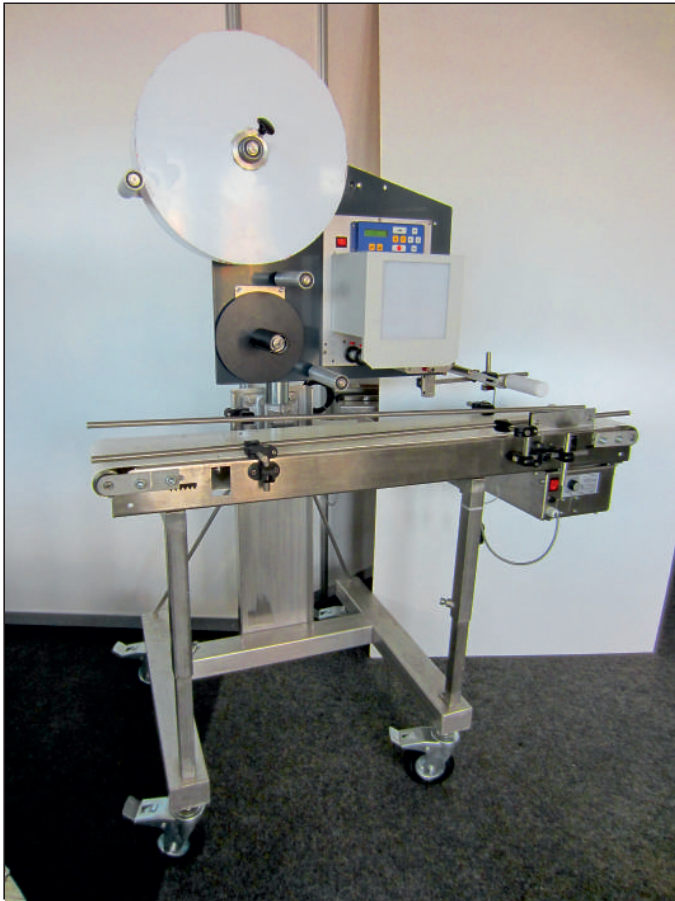
Labelling station with dispenser, printer and conveyor
